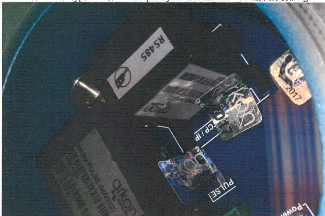
Figure 2: The water meter type MAGX2 – frequency module and RS 485 module sealing:
