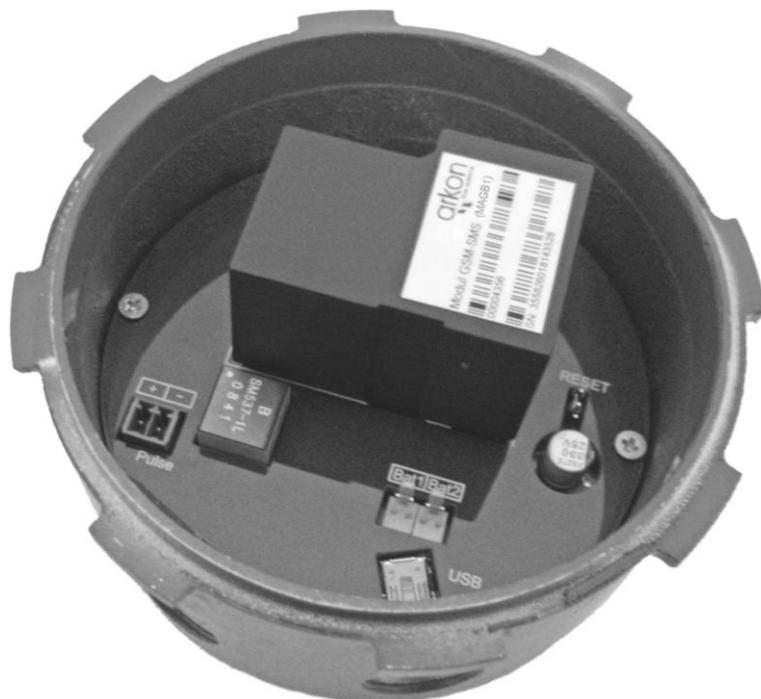
Picture 3. Install GPRS/GSM Module into the transmitter
