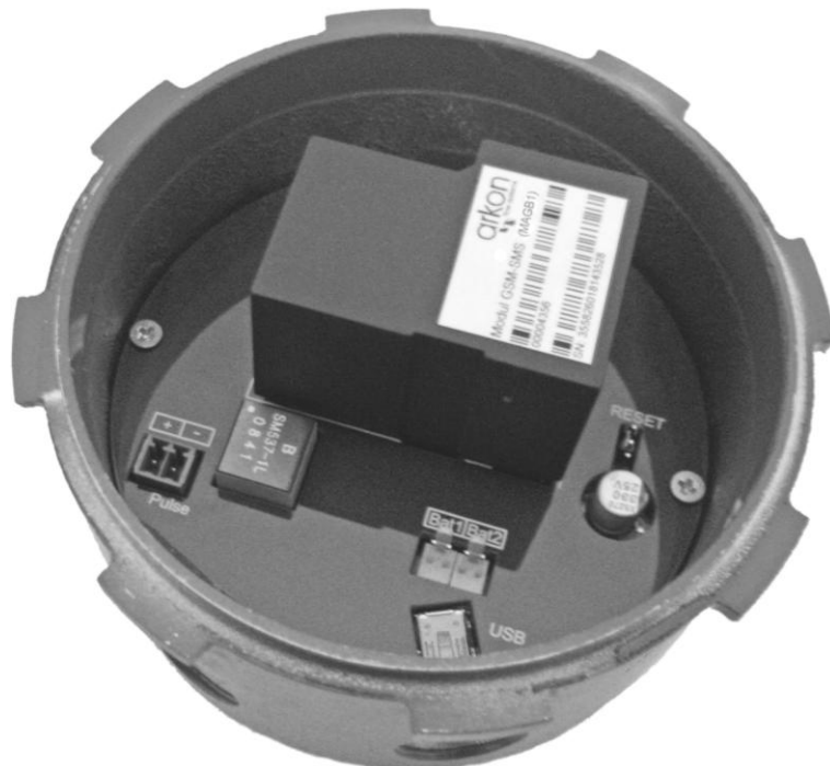
Picture 3. Install GSM-SMS Module into the transmitter
