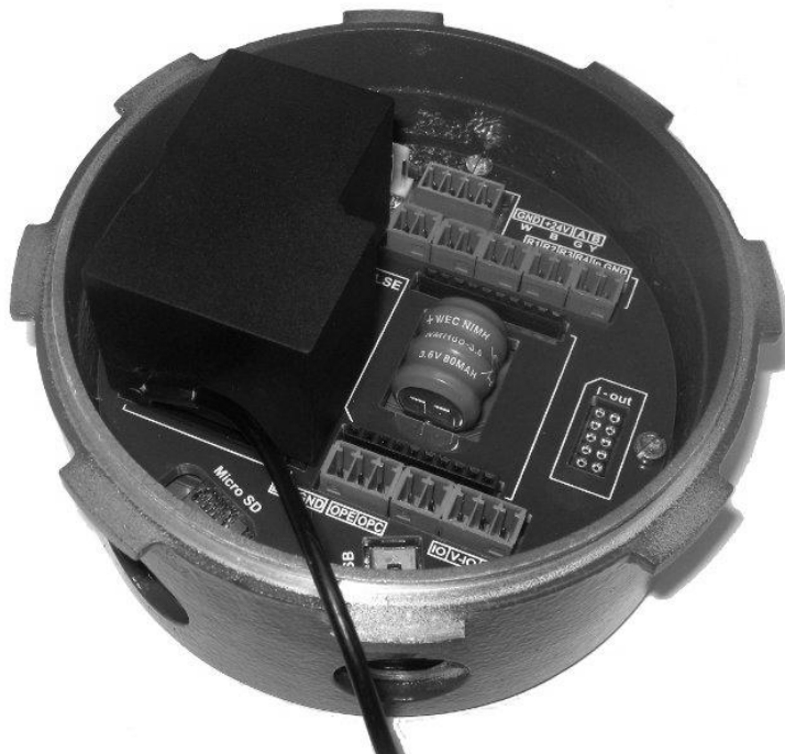
Picture 3. Install GSM SMS Module into the transmitter
